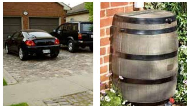
Installing permeable pavers (as opposed to asphalt or concrete) and rain barrels are two methods residents can adopt to help reduce runoff to storm sewers.
